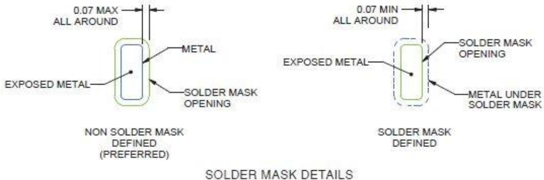
LAND PATTERN EXAMPLE EXPOSED METAL SHOWN SCALE:12X
