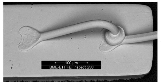
The PCB pad is covered by ENIG: Ni can be detected through the Au.
