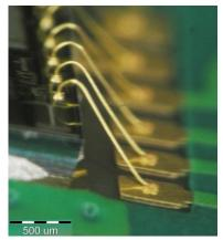
Usually thermosonic ball bonds are made to AI contact pads of the IC or sensor chips. Optical microscopic photos and SEM (Scanning Electron Microscopic) images provide good possibilities to study the structures of the bonds.
